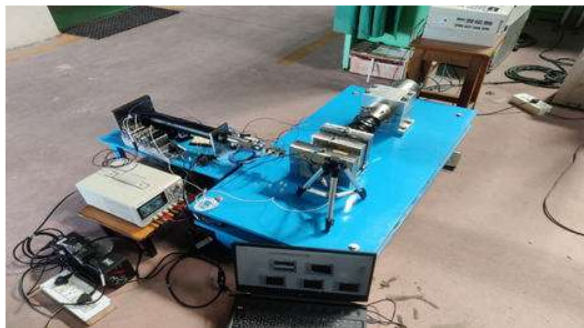
Test rig for high speed bearing noise measurement
