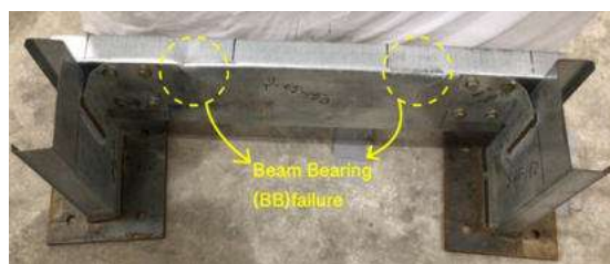
Beam bearing failure.
